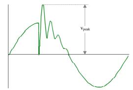
Figure 4: Characterisation of oscillatory transient
