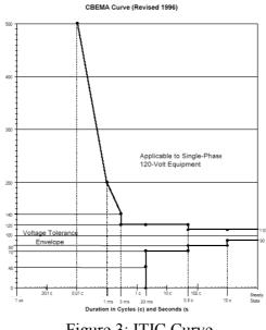
Figure 3: ITIC Curve
