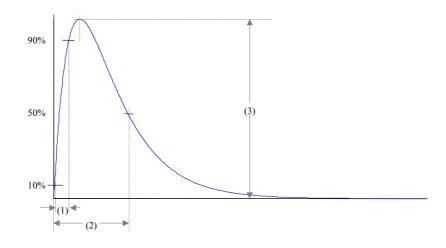
Figure 5: Characterisation of impulsive transient
